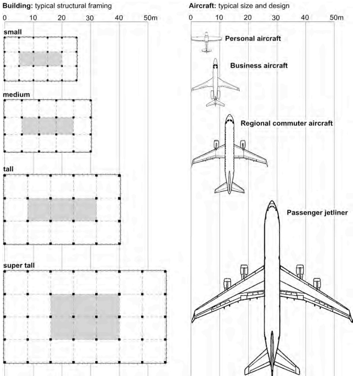
Figure 17: Representative structural framing and typical aircraft size
