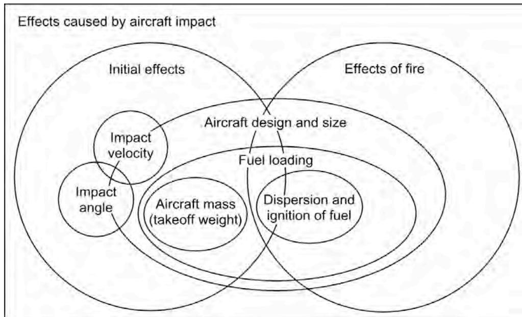
Figure 8: Aspects of the effects caused by aircraft impact on buildings
