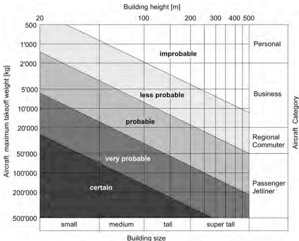
Figure 20: Probability of building collapse due to aircraft impact depending on aircraft and building size
