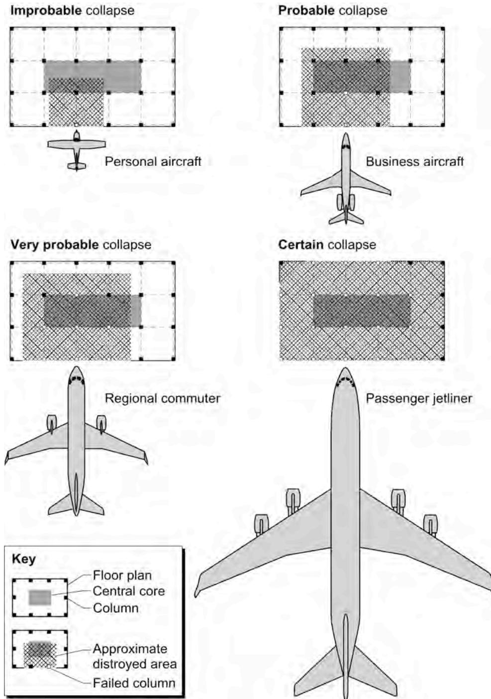
Figure 18: Structural damage and probability of building collapse for medium size high-rise buildings
