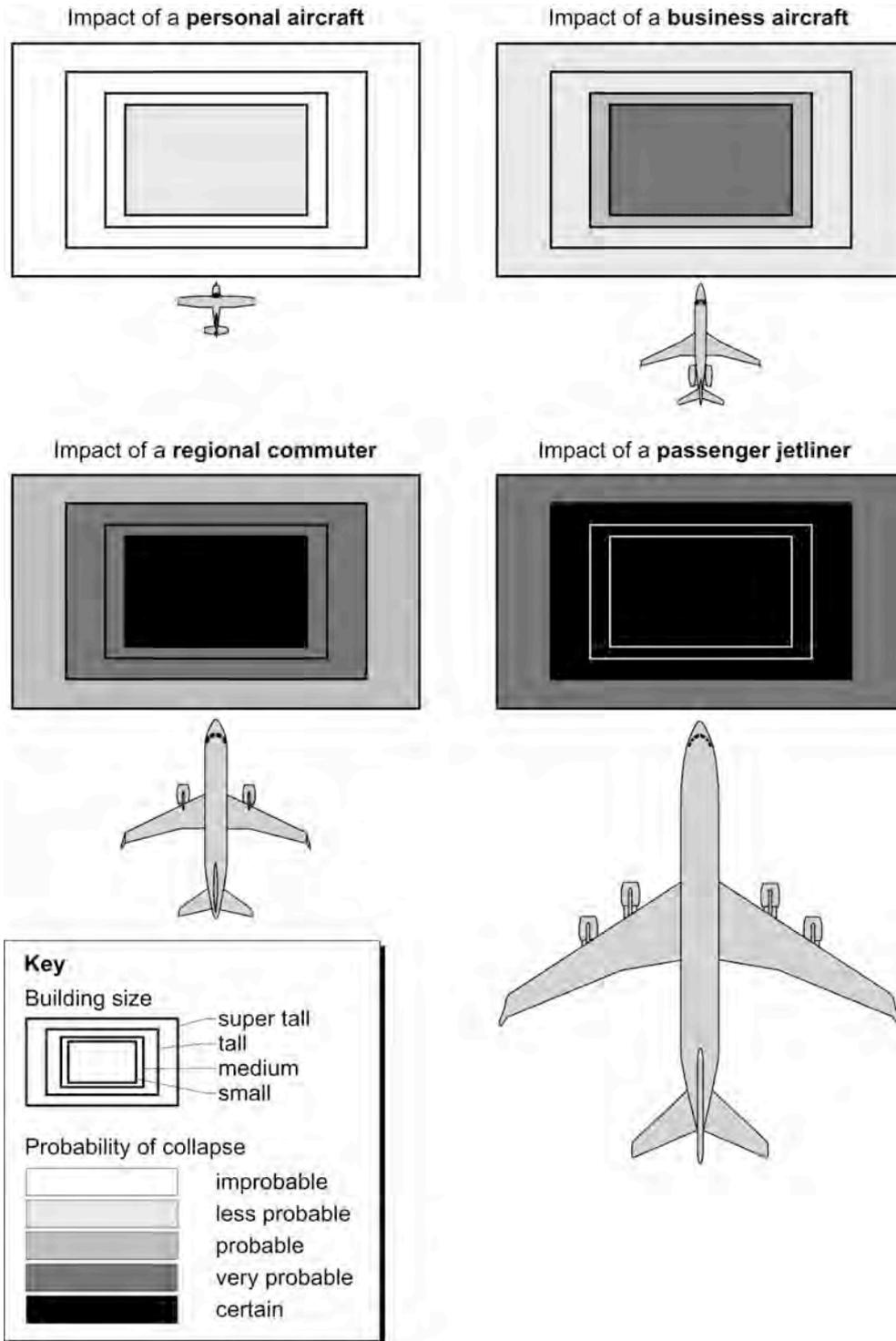
Figure 19: Probability of building collapse caused to aircraft impact
