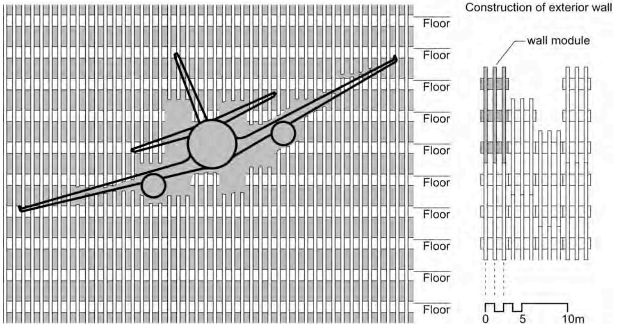
Figure 6: Impact damage to exterior columns of WTC 1 (left) and construction of the exterior wall with modules (right)
